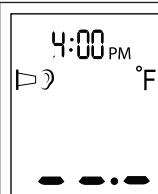
2. Press and hold the ON/OFF button for three seconds; "MEM" and the last stored measurement will appear on the LCD Display.
