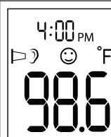
3. To view stored measurements, press the ON/OFF Button to cycle; the memory number is displayed first followed by the measurement.
